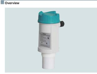
SITRANS LU180 is a short-range integrated ultrasonic level transmitter. It is intrinsically safe (ATEX, CSA, FM, IECEx, NEPSI), 2 wire, 4 to 20 mA loop powered, ideal for liquids, slurries, and bulk materials in open or closed vessels to 5 meters (16.4 feet).
